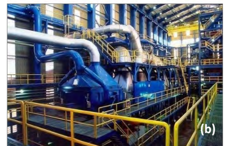
CBMM's operations: (a) open pit mine and (b) sintering unit at the ferroniobium plant (Photos: Courtesy of CBMM)
